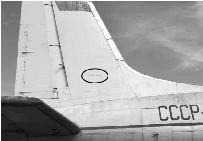
The Il-18 construction number is often painted on the tail and also to be noted on the forward underside of the wing, close to the fuselage.
