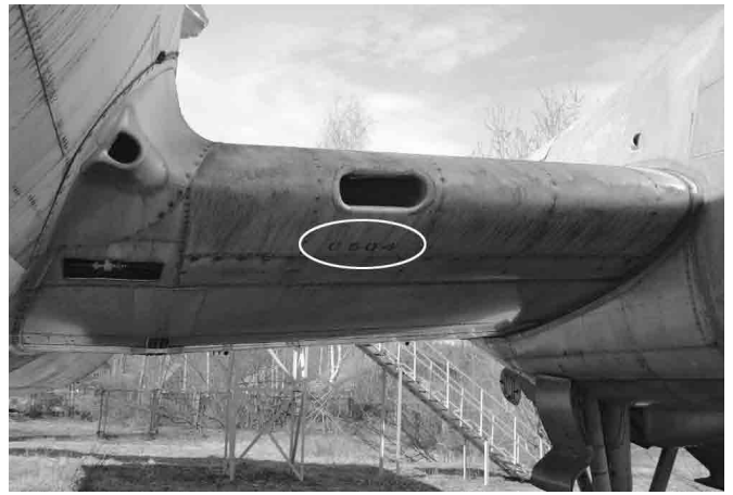
The Il-18 construction number is often painted on the tail and also to be noted on the forward underside of the wing, close to the fuselage.
