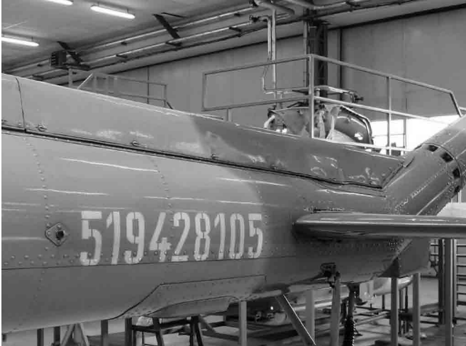
The construction number is normally painted on both sides of the tail boom. Preferably the plate has to be checked and this is to be found on the right side of the cockpit instrument panel and is easily readable from the outside.
