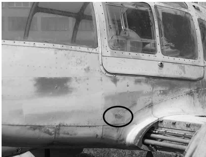
The construction plate is at the left side of the lower fuselage just in front of the wing root.
