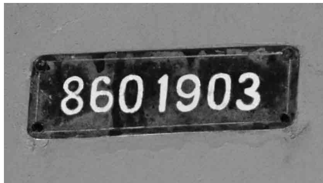
The construction number (or just its last five digits) is normally found in the nose wheel bay.
