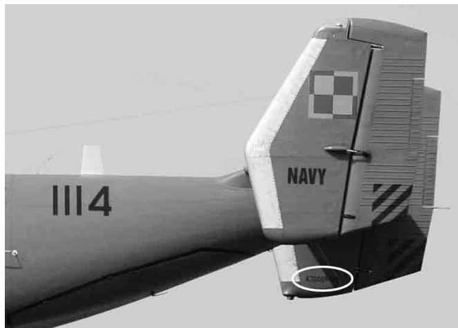
The construction number is often painted on the inside of both vertical stabilizers. The construction number plate is found under the horizontal tailplane on the left side.
